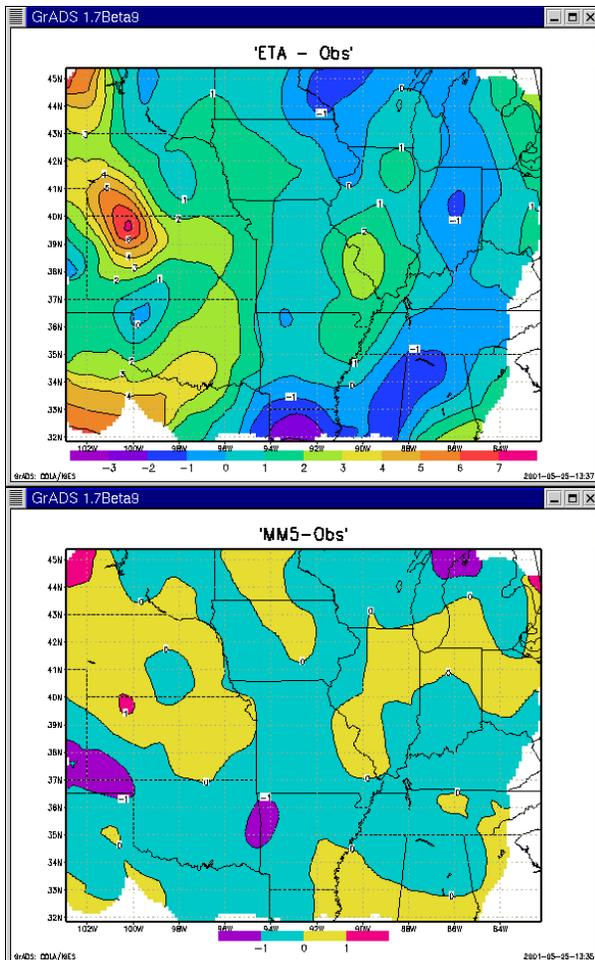
Fig. 2. Difference ( $^{\circ}\text{C}$ ) between lowest sigma-level temperature and observed 2 m temperature from MM5 initialization at 12 UTC 24 May 2001 for 1) initialization with Eta analysis only and b) initialization with Eta analysis, surface observations and sounding.
