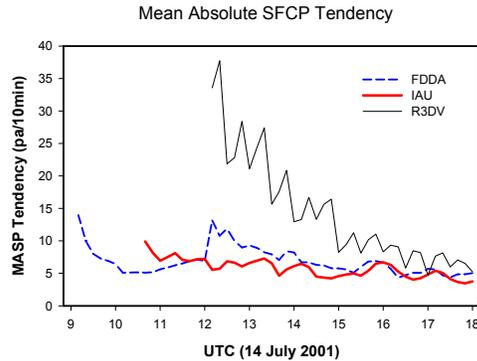
Fig. 2 Absolute tendency of surface pressure averaged over the model by 3DVAR system without IAU as a control (R3DV in thin line) and with IAU (thick line), and by 3hr nudging (dashed line).
