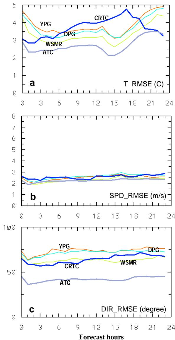
Fig. 8 Domain-average of RMSE errors of WRF surface temperature (a), wind speed (b) and wind direction (c) forecasts on the domains centered at 5 Army test ranges, between March 04 and 18, 2004.
