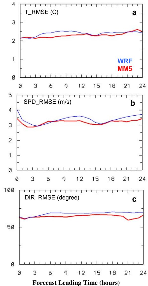
Fig. 2 Domain average of RMSE errors of the surface temperature (a), wind speed (b) and wind directions (c) forecasts of WRF (thin-blue) and MM5 (thick-red) with respect to forecast time, for the 28 forecast days in the April and May, 2004.
