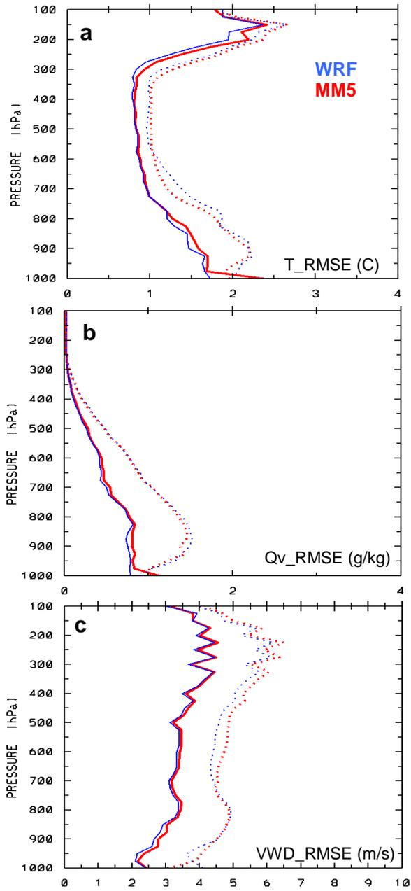
Fig.4 Domain-average RMSE errors of upper-air temperature (a), specific humidity (b), and vector wind differences (c) of WRF (thin-blue) and MM5 (thick-red) 0-h (solid) and 12-h forecasts (dotted) for the 28 forecast days in the April and May, 2004.
