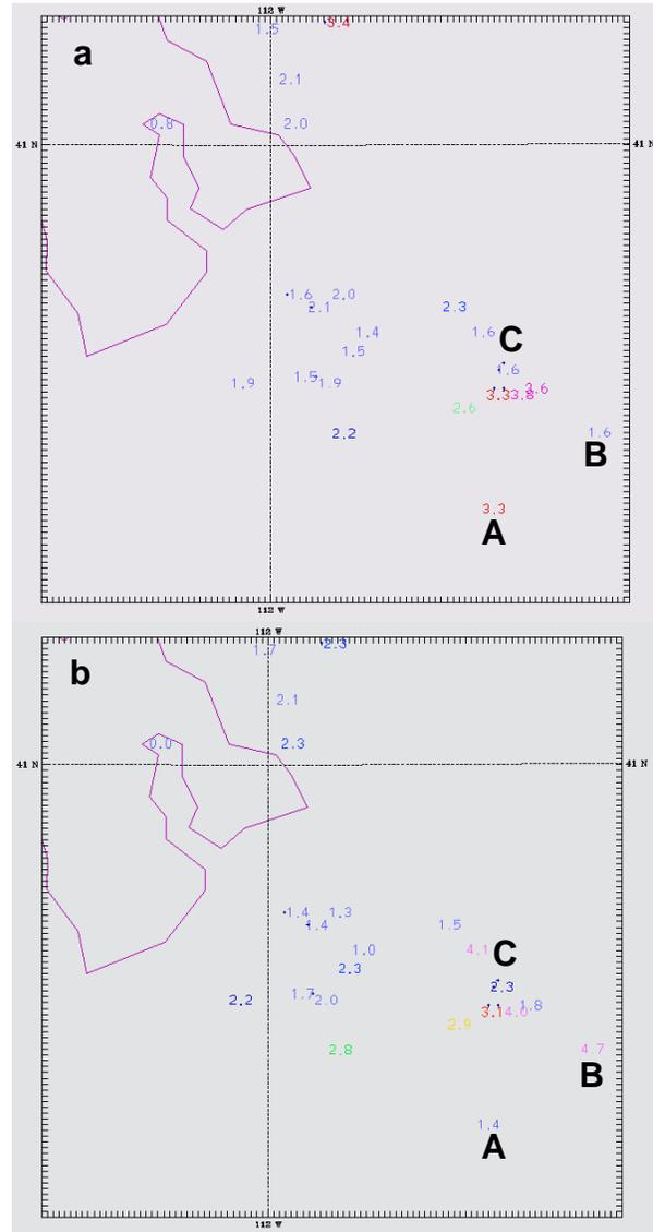
Fig. 7 Surface temperature RMSE errors (C) at available observations stations of the 18-h MM5 (a) and WRF (b) forecasts, valid at 18Z and averaged for a 14 forecast days between May 9 and 23, 2004.
