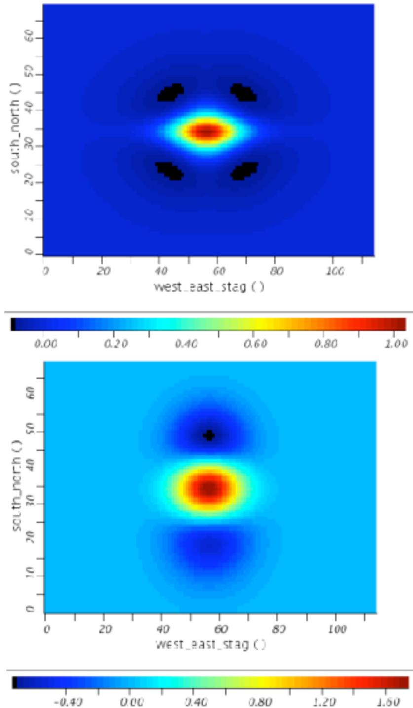
**Fig. 1:** U-Wind horizontal analysis increment structure due to the assimilation of a single u-wind observation (difference from first-guess = 2m/s). Upper (NCAR/UKMO BE model), lower (NCEP BE model).
