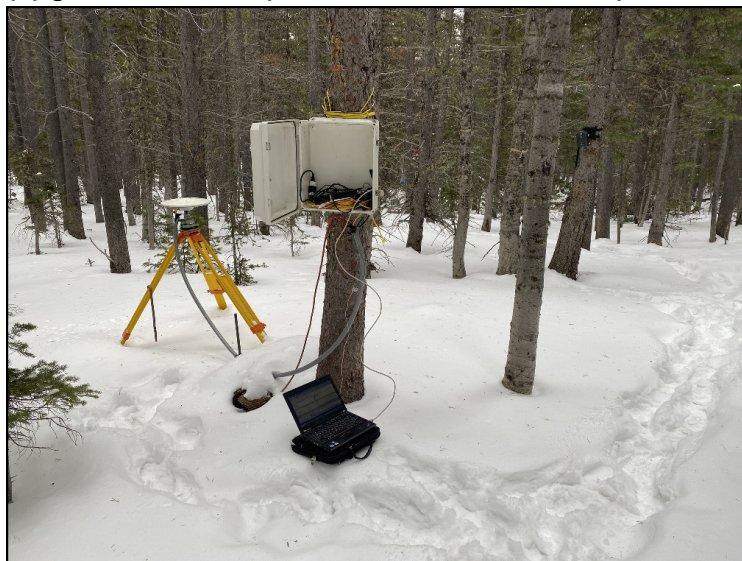
Figure S1. Photos of (a) the gnssA antenna at the top of the US-NR1 26-m tower, and (b) the gnssB antenna mounted on a tripod above the forest floor. The white enclosure shown in (b) , housed the gnssB receiver and the photo is taken northwest of the antenna so that the trees south and southeast of the antenna are shown.
