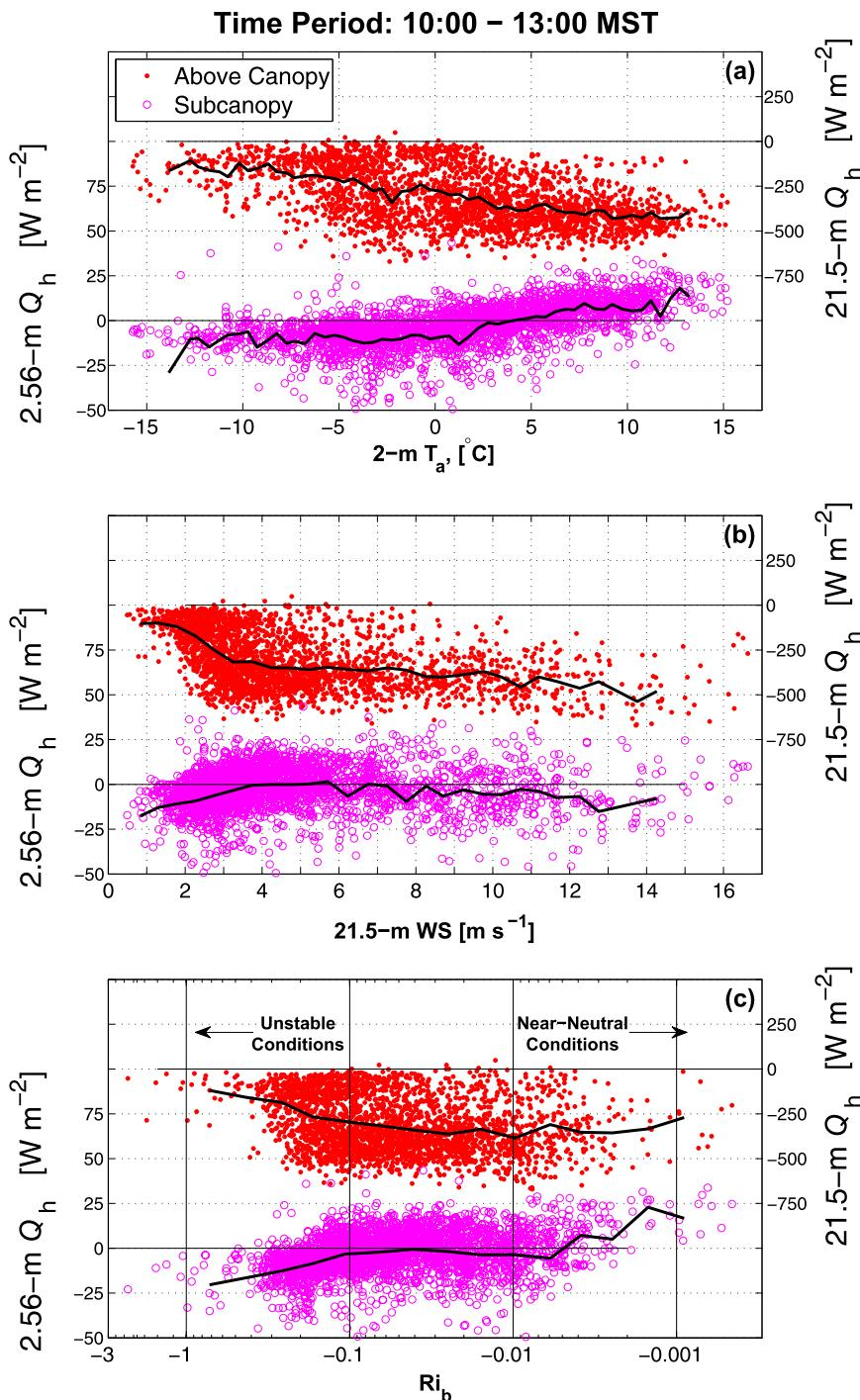
FIG. 9. The subcanopy (left axis) and above-canopy (right axis) sensible heat flux  $Q_h$  as a function of (a) 2-m air temperature  $T_a$ , (b) 21.5-m wind speed WS, and (c) bulk Richardson number  $Ri_b$ . These data are from 1000 to 1300 MST for March and April between years 2005 and 2010, and the black line is the binned mean of the 30-min values.
