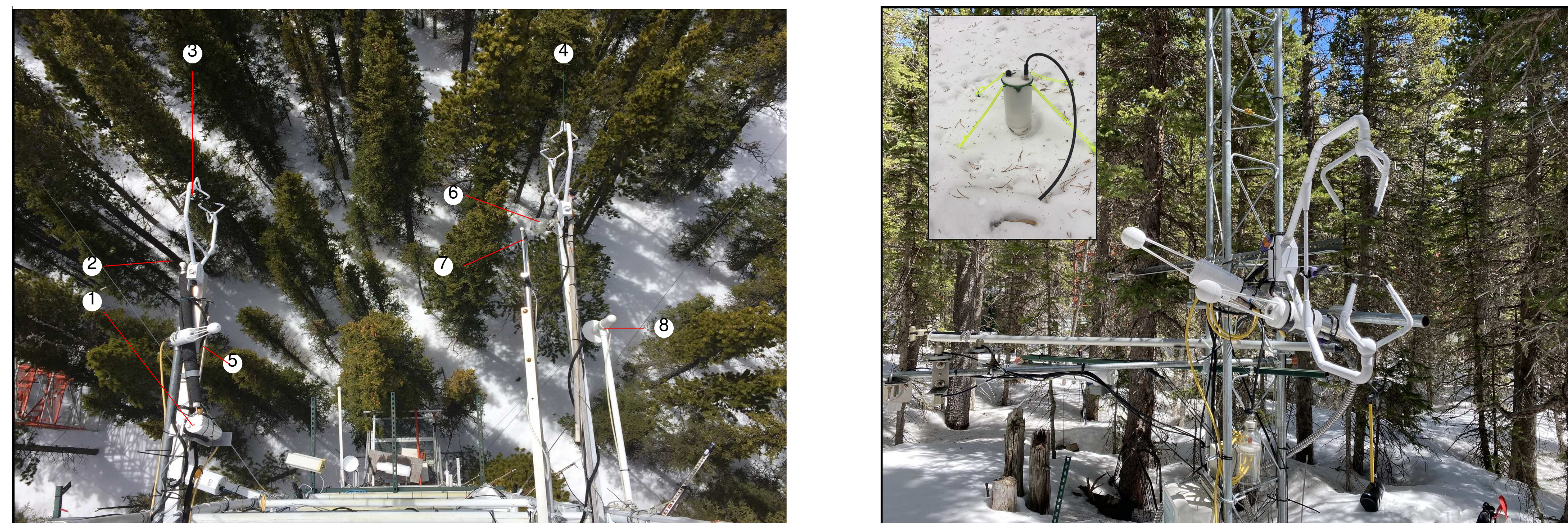
Figure 1: Photographs of the instrumentation at the US-NR1 AmeriFlux site, (left) looking down at the instrumentation deployed at 21.5 m and (right) the subcanopy flux sensors deployed at 2.5 m (photo inset: an EOS FD Sensor as snow starts to accumulate). The numbered instruments are: ① LI-COR LI-7200 body, ② LI-7200 inlet, ③ and ④ CSI CSAT3s, ⑤ LI-COR LI-7500A, ⑥ LI-6262 inlet, ⑦ Krypton Hygrometer, and ⑧ Vaisala T7RH
