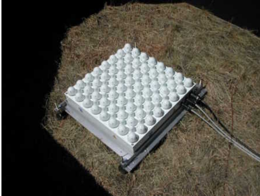
Figure 4-3. Scintec Model MFAS SODAR antenna
