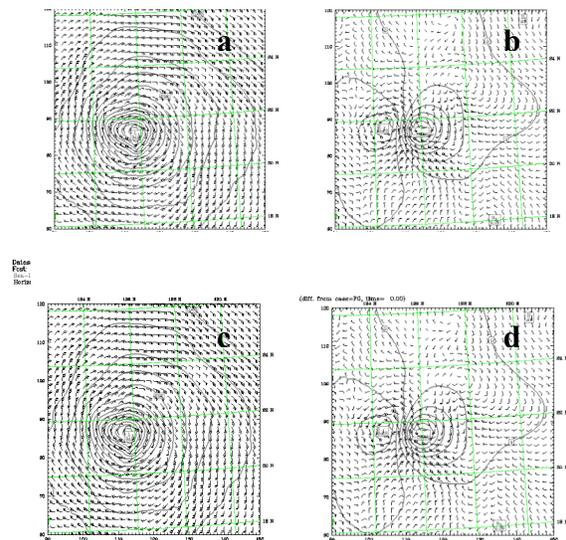
Fig. 5. Analysis of Typhoon Haitang a) SLP and surface wind fields and b) increment of SLP and wind from 3DVCV5E3, c) SLP and surface wind fields and d) increment of SLP and wind from 3DVCV5E2.
