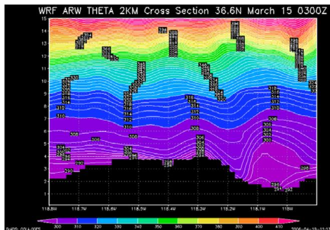
**Figure 2.** WRF-ARW (2 km resolution) 15-h forecast of W-E vertical cross-section including southern Owens Valley in IOP4, 03 UTC Mar 15 2006, showing potential temperature isentropes kinking to lee of Sierra Nevada and hinting at a transition from trapped lee wave to lee downslope wind event.
