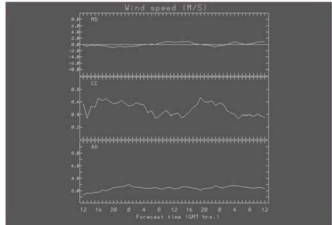
**Figure 1.** Wind speed mean differences (bias), correlation coefficients, and mean absolute differences compiled for all DRI mesonet sites by each forecast hour, during the Mar-Apr 2006 T-REX period.
