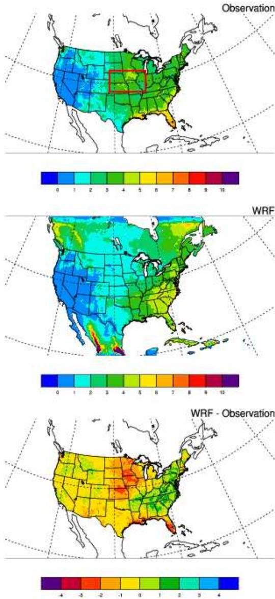
Figure 1: 6-Year warm-season average daily rainfall (mm) for (top) 1/24° gridded observations, (middle) WRF model and (bottom) the difference (model - observation). The red-box in (top) indicates the flood region over which area average rainfall values are taken.
