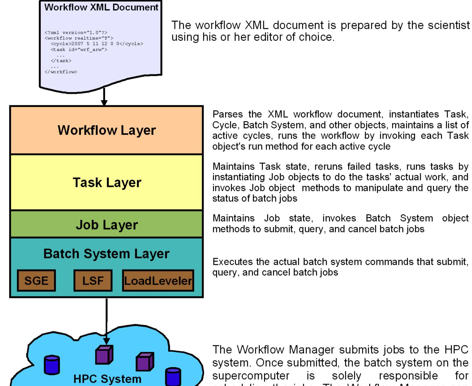
Parses the XML workflow document, instantiates Task, Cycle, Batch System, and other objects, maintains a list of active cycles, runs the workflow by invoking each Task object's run method for each active cycle
