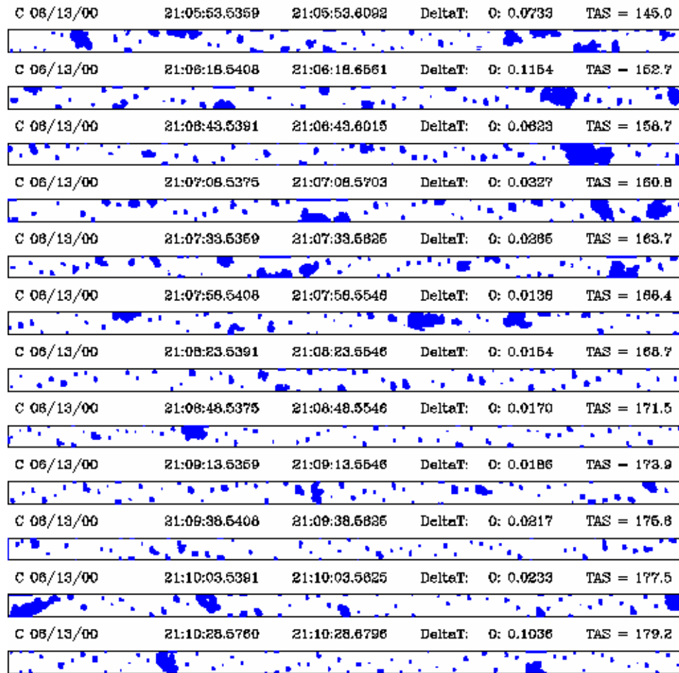
Figure 3.7 Buffers of particles imaged by the 2-DC probe. The vertical dimension of each row is ~ 1mm. Text across the top of each buffer designates flight day (M/D/Y); start time of first image in that buffer (row); start time of last image in the buffer; DeltaT: = elapsed time to fill the buffer; TAS = true airspeed of the aircraft. The TAS is used to determine the horizontal particle size.
