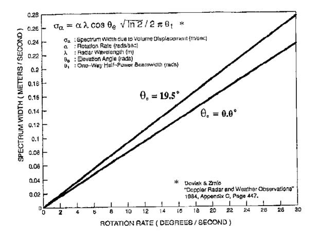
Figure A-1. NEXRAD SPECTRUM WIDTH DUE TO VOLUME DISPLACEMENT
