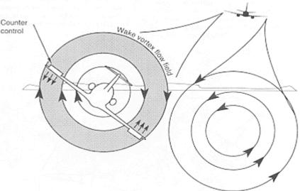
Differential pressure field above and below wing generated by the vortices causes roll up
