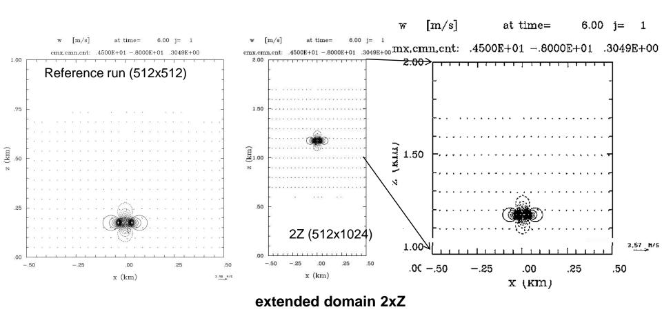
Cyclic BC: vortex propagation speed highly sensitive to treatment at boundary
