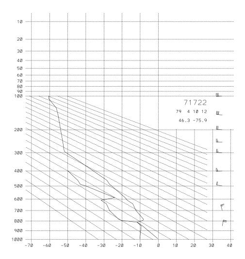
Fig. 4.2: Sample sounding plot (Stüve diagram), showing vertical distribution of temperature, dewpoint, and wind. The sloping dashed lines are lines of constant potential temperature. The vertical pressure coordinate is scaled by  $p^{\kappa}$ , where  $\kappa = \frac{2}{7}$ . Plots are generated by RAWINS and written to the file SND.PLT.
