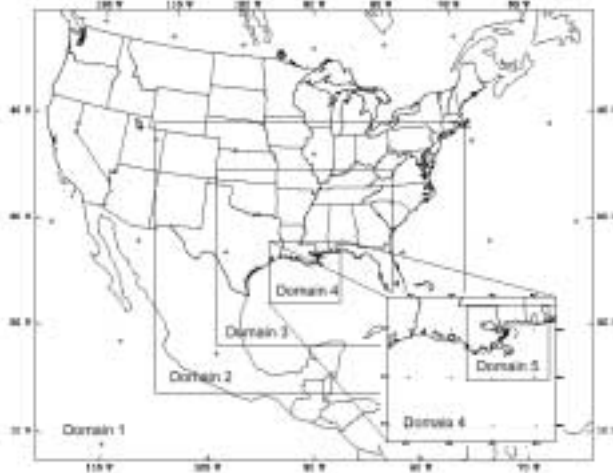
Fig. 1. The domains for the five MM5 grid meshes used in this study: Domain 1 (81 km), 2 (27 km), 3 (9 km), 4 (3 km), and 5 (1 km). The first three domains were integrated using two-way interactive mode. The 3 km and 1 km grids were integrated with one-way nesting.
