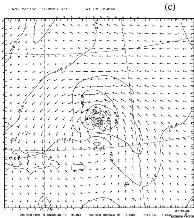
Figure 1. 1000 hPa wind field (cont 5  $\text{ms}^{-1}$ ) of (a) first guess, (b) background, and (c) final field after bogussing hurricane floyd valid at 0000 UTC Sept 12 1999.
