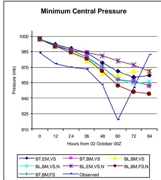
Fig. 2: Minimum central pressure on the 30 km grid vs. hours into simulation and observed values for Hurricane Opal.
