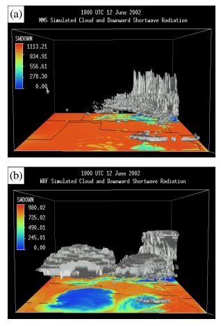
Figure 4. Simulated liquid cloud water (mixing ratios greater than .0001 kg/kg shown in white isosurfaces) and downward shortwave radiation flux ( $W m^2$ ) at the surface (shown in colored horizontal field) valid at 1800 UTC 12 June 2002 for the (a) MM5 simulation and the (b) WRF simulation.
