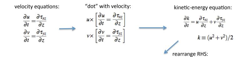
$$\frac{\partial k}{\partial t} = \underbrace{\left(\frac{\partial (u\tau_{xz})}{\partial z} + \frac{\partial (v\tau_{yz})}{\partial z}\right)}_{\text{diffusion}} - \underbrace{\left(\tau_{xz}\frac{\partial u}{\partial z} + \tau_{yz}\frac{\partial v}{\partial z}\right)}_{\text{dissipation }(\varepsilon)}$$
