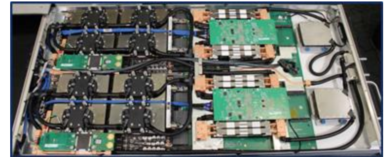
Above: A Derecho GPU blade with two GPU nodes, each with 1 AMD EPYC Zen3 “Milan” 64-core processor and 4 NVIDIA A100 Ampere GPUs.
