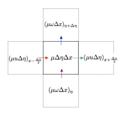
Mass in a control volume  $(\Delta x \Delta \eta)(\mu)^t$ Scalar mass  $(\Delta x \Delta \eta)(\mu \phi)^t$
