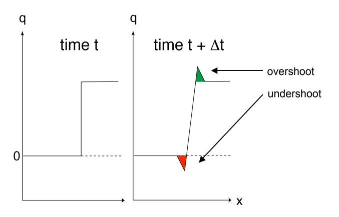
ARW scheme is conservative, but not positive definite nor monotonic. Removal of negative q results in spurious source of q .
