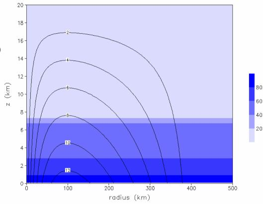
colors = relative humidity (%) contours = azimuthal velocity (m/s)
