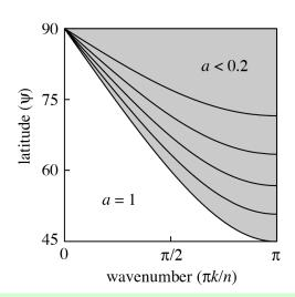
Converging gridlines severely limit timestep. The polar filter removes this limitation.
