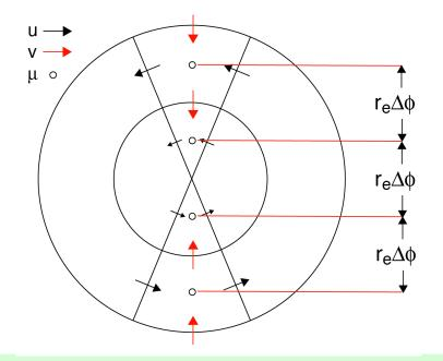
Zero meriodional flux at the poles (cell-face area is zero).
