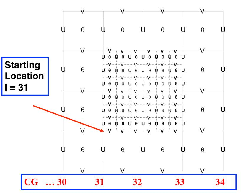
Coarse Grid Staggering 3:1 Ratio
