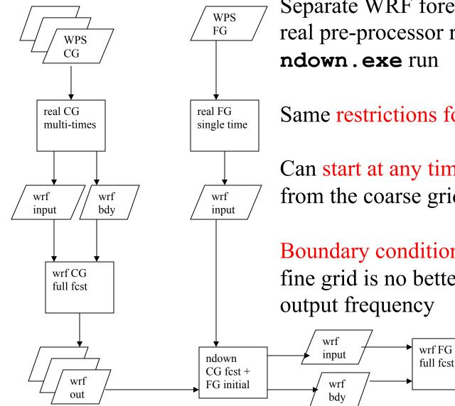
Separate WRF forecast runs, separate real pre-processor runs, intervening **ndown.exe** run
