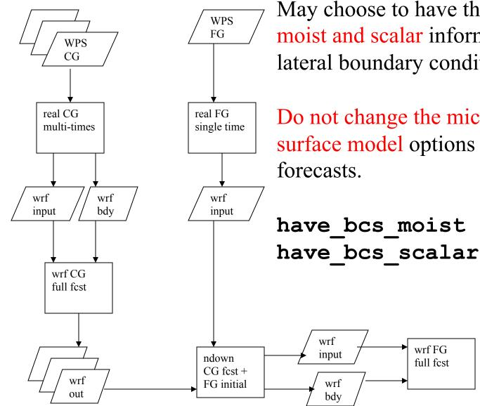
May choose to have the parent WRF model moist and scalar information used for the lateral boundary conditions.
