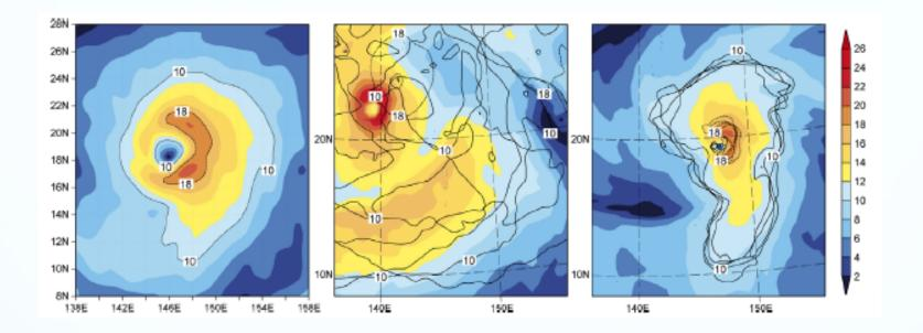
Horizontal 10 m wind speed fields (m s-1) for typhoon Songda (200418), on 1 September 2004, 0:00.
