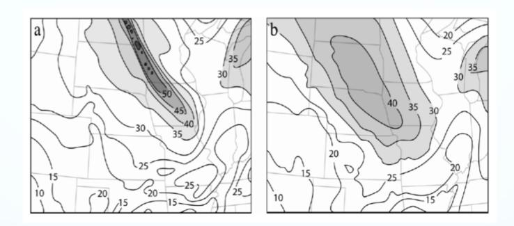
12-hour simulations of 250-hPa winds (m s-1) from the 40-km grid increment Eta Model initialized at 1200 UTC 3 August 1992, based on experiments that used a large (a) and a small (b) computational domain. (Warner, 2011)
