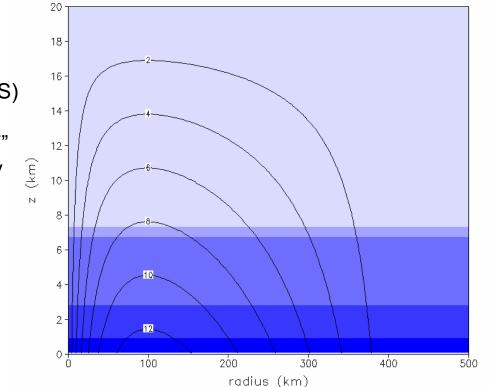
colors = relative humidity (%) contours = azimuthal velocity (m/s) 80
