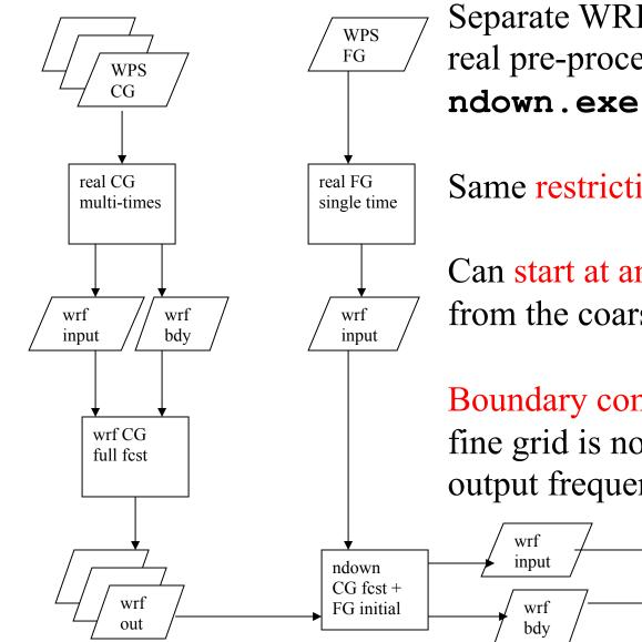
Separate WRF forecast runs, separate real pre-processor runs, intervening **ndown.exe** run
