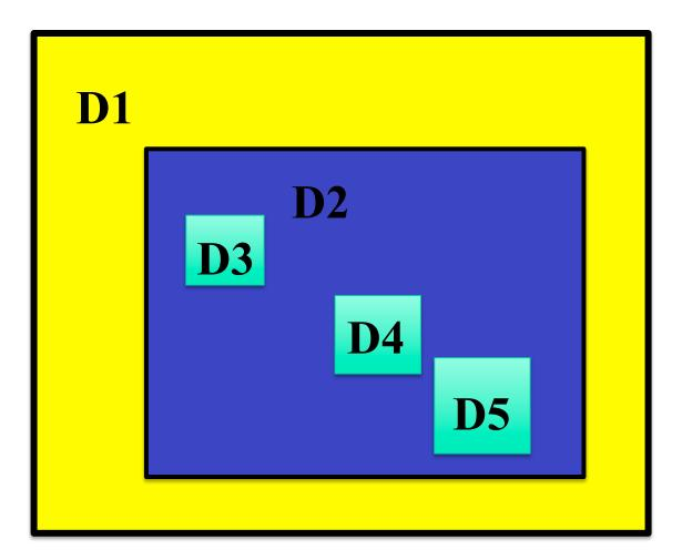
WRF 5-domain run: Domain 1 (a single 3 min dt), then Domain 2 (a single 1 min dt). Then Domain 3, in 20 s pieces up to 1 min. Then Domain 4, in 20 s pieces up to 1 min, and same with Domain 5.
