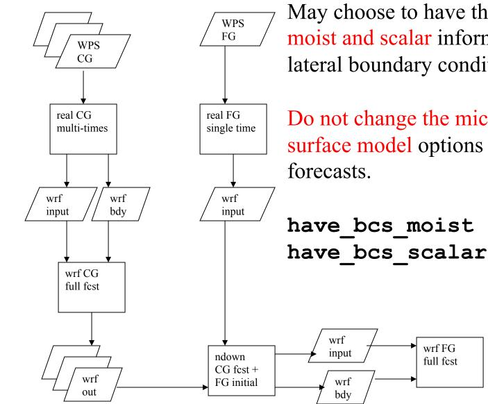
May choose to have the parent WRF model moist and scalar information used for the lateral boundary conditions.
