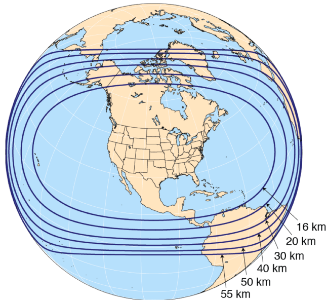
Above: An MPAS 60-15 km variable-resolution mesh with refinement over North America
