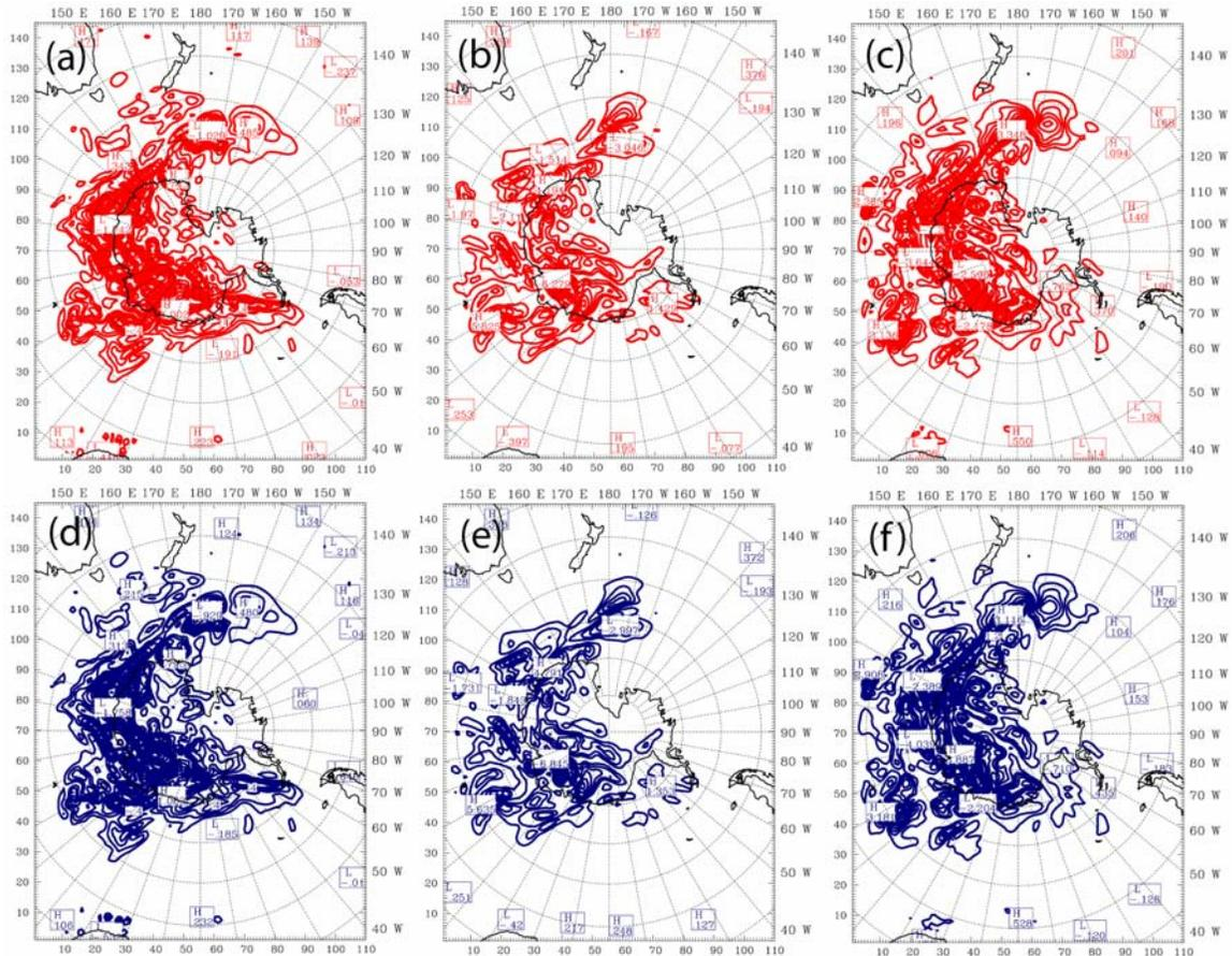
Fig. 5: The difference of (a) potential temperature, (b) u component and (c) v component of wind between two parallel WRF\_SN runs and the increment of (d) potential temperature, (e) u component and (f) v component of wind by WRF tangent linear model integration at 500 hPa at 0000 UTC 16 May 2004 (24-h forecast)
