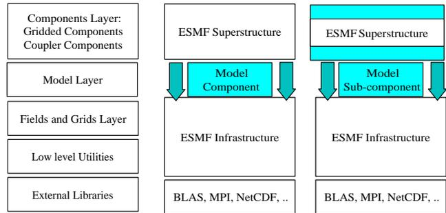
Figure 1: Structure of a coupled ESMF application
