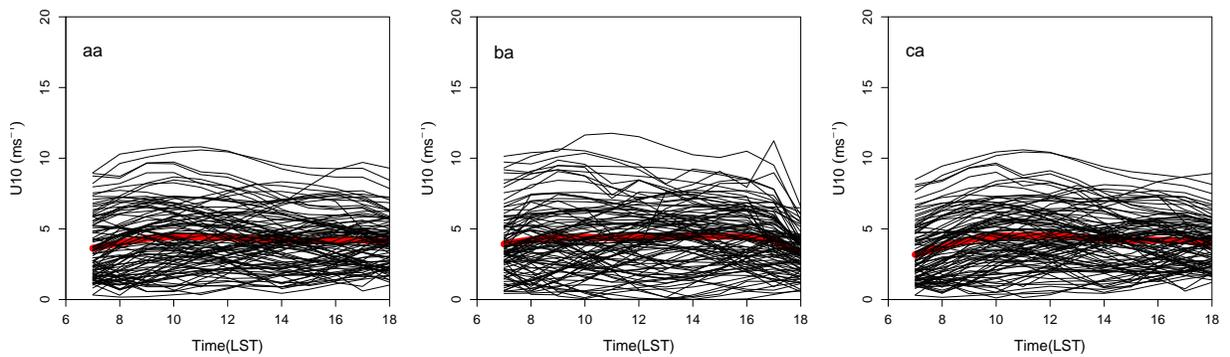
Figure 4: Daytime individual ensemble members (black) and ensemble mean (red) 10-m wind speed for different boundary layer schemes (first label letter): a – YSU, b – MRF c – MYJ with a – NOAH LSM (second label letter).
