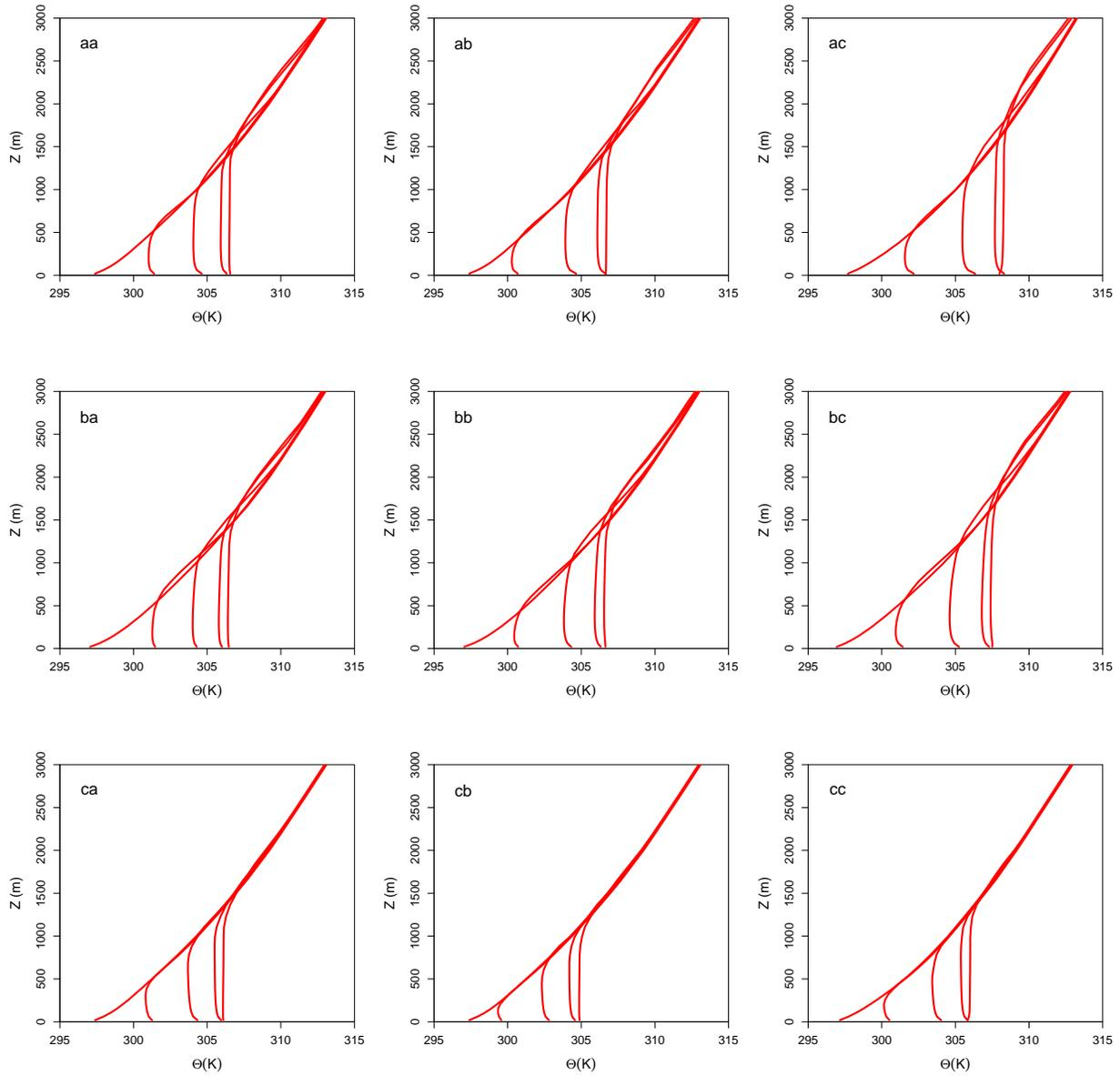
Figure 1: Mean vertical profiles of potential temperature at 06, 09, 12, 15, and 18 LST for different boundary layer schemes (first label letter): a – YSU, b – MRF, c – MYJ and land-surface schemes (second label letter): a – NOAH, b – RUCLSM, c – SLAB.
