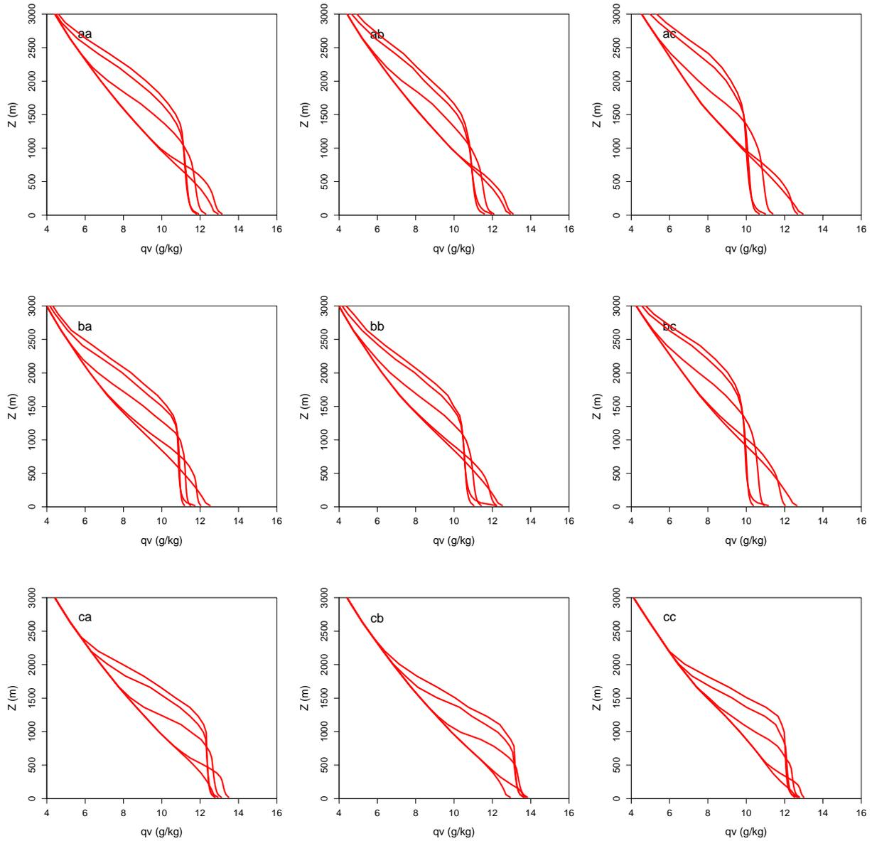
Figure 2: Mean vertical profiles of mixing ratio at 06, 09, 12, 15, and 18 LST for different boundary layer schemes (first label letter): a – YSU, b – MRF, c – MYJ and land-surface schemes (second label letter): a – NOAH, b – RUCLSM, c – SLAB.
