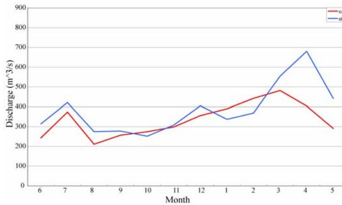
Figure 6 Comparison of 10-year average monthly mean discharge between observation in the 1990s and calculation in the 2070s.
