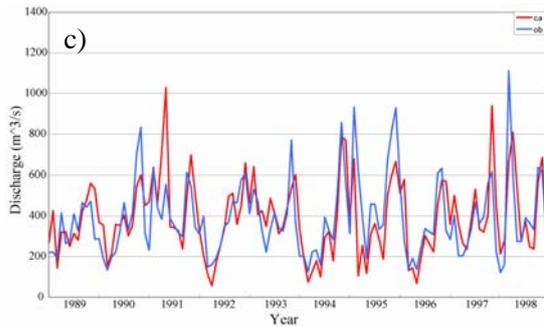
Figure 4 Comparison of monthly mean discharge in the 1970s (a), 1980s (b) and 1990s (c) between observation and calculation.
