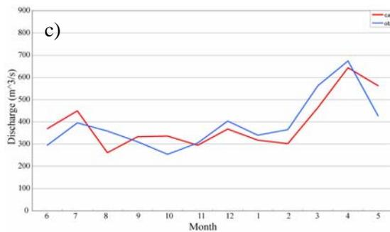
Figure 5 Comparison of 10-year average monthly mean discharge in the 1970s (a), 1980s (b) and 1990s (c) between observation and calculation.
