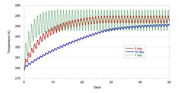
Deep soil temperature response to different deep soil timescales
