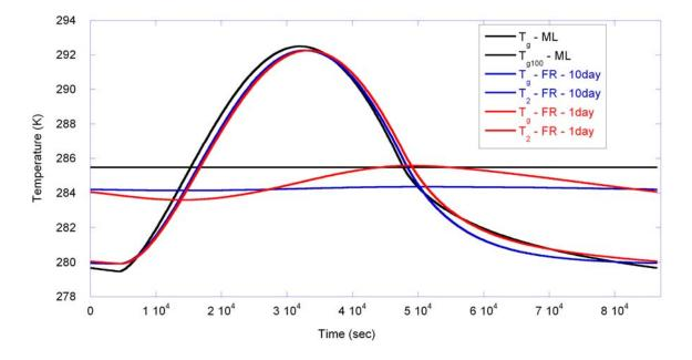
Force-Restore vs 100-layer model for realistic surface forcing
