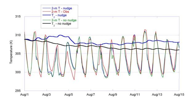
Comparison of T-2m and deep soil T with and without deep soil temperature nudging for a single grid cell in south Texas
