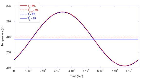
Force-Restore vs 100-layer model for sinusoidal surface forcing
