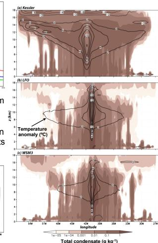
The warmer, and larger radial gradient of  $\bar{T}_v$  in the Kessler storm results from a much more prominent anvil than in either of the two ice MP storms (right). This is the opposite of squall line simulations because of the much weaker mean updraft speed in TCs, less condensation, and slower conversion of cloud droplets to rain drops in the Kessler scheme.
