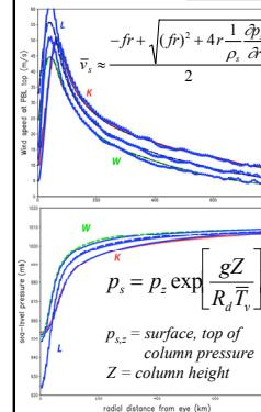
Hydrostatic balance also does an excellent job of replicating the radial distribution of  $p_s$  in the vortex (bottom left). Here  $Z=14.5$  km, a height where  $p_s$  does not vary much among the cases, and thus  $\bar{T}_v$  (below, middle) controls the surface pressure differences between the runs.
