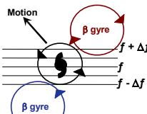
In the absence of environmental steering flow, the motion of a TC results from "ventilation flow" across the vortex from beta gyres, which owe their existence to differential advection of planetary vorticity by the TC. The strength of the wind field at large radii controls the strength and orientation of the gyres and thus the direction of storm motion.
