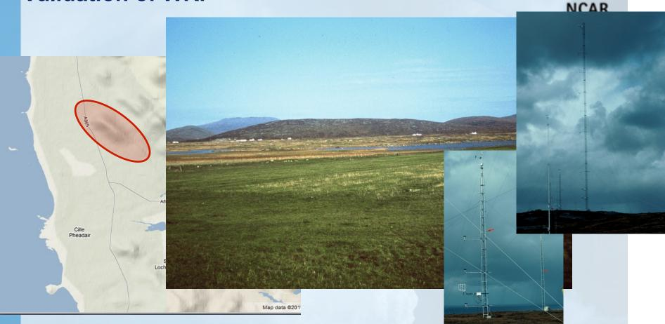
Askervein Hill experiment took place on the West side of South Uist island (Scotland) in 1983 (Taylor and Teunnisen, BLM 1987). Measurements were taken using cup anemometers mounted at 10m above the ground on 50 towers.
