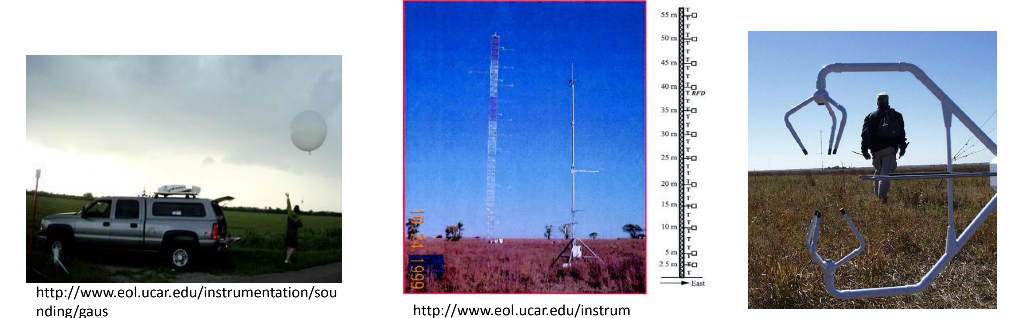
Fig. 5 Pictures of observation instruments: sounding (left), tower (middle), and sonic anemometer (right).
