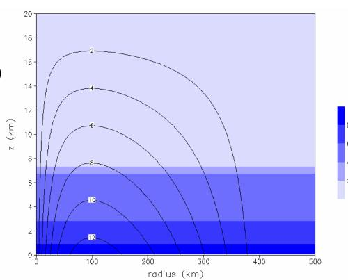
colors = relative humidity (%) contours = azimuthal velocity (m/s)
